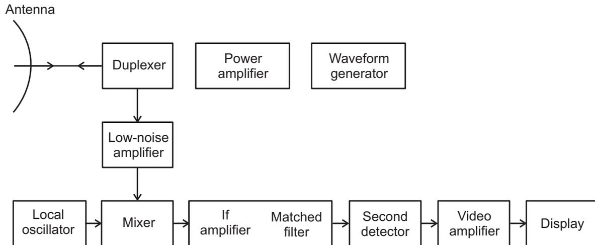
Figure 1: Block Diagram of Elementary RADAR system
